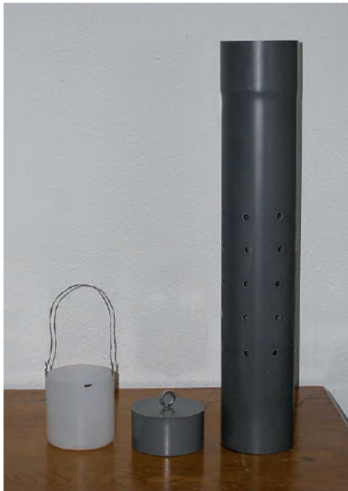
Fig. 10. Assembled main components of a MSS trap (© MNCN; photographer: M.A. Alonso-Zarazaga).
