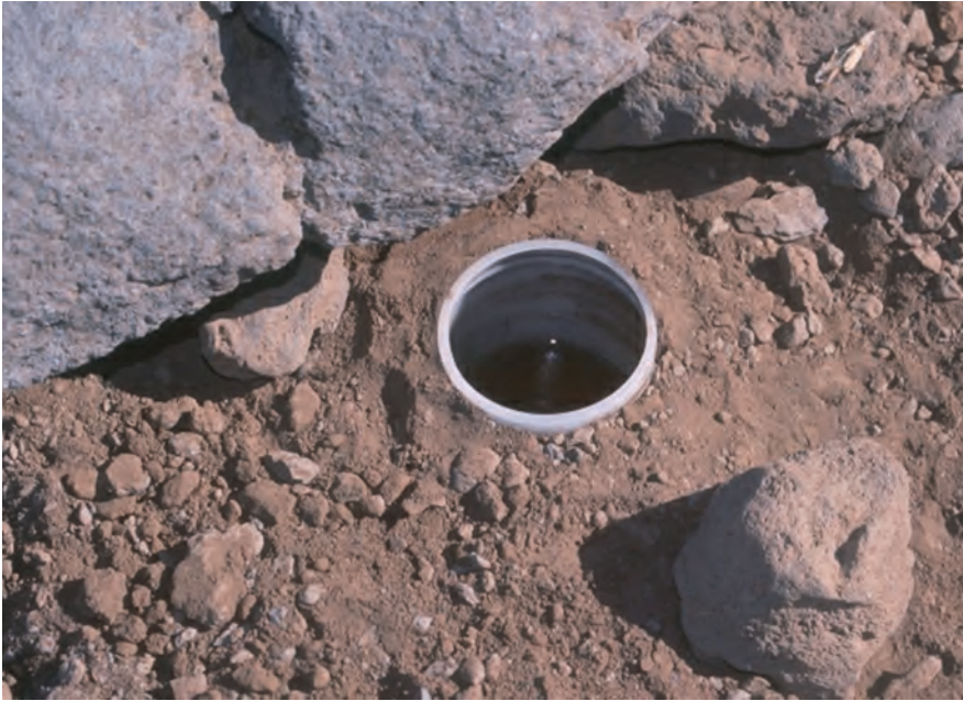
Fig. 4. Pitfall trap from outside, ready to work, showing its rim flush with the ground surface and ethylene glycol solution inside (© MNCN; photographer: Antonio Sánchez-Ruiz).
