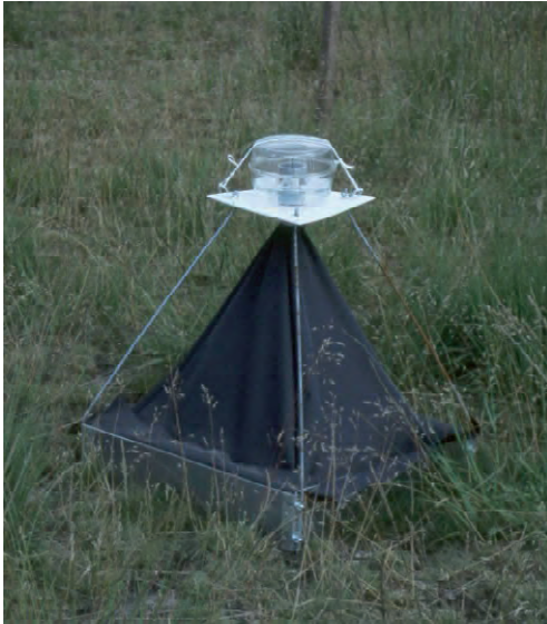
Fig. 6. Emergence trap in the field. The collecting jar is a plastic commercial wasp trap filled with 70% alcohol. (Photo by Wouter Dekoninck).
