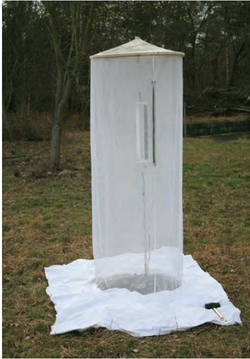
Fig. 4. Personal light-trapping. Two battery-powered 15 W fluorescent tubes in a gauze cylinder ("tower"). (Photo by A. Steiner).
