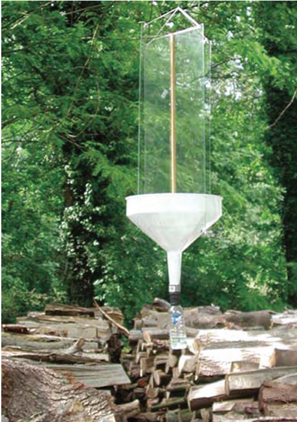
Fig. 28. Suspended Perspex quadrilateral window-pane interception trap with a collecting bottle at the bottom. (Photo by B. Mériquet).
