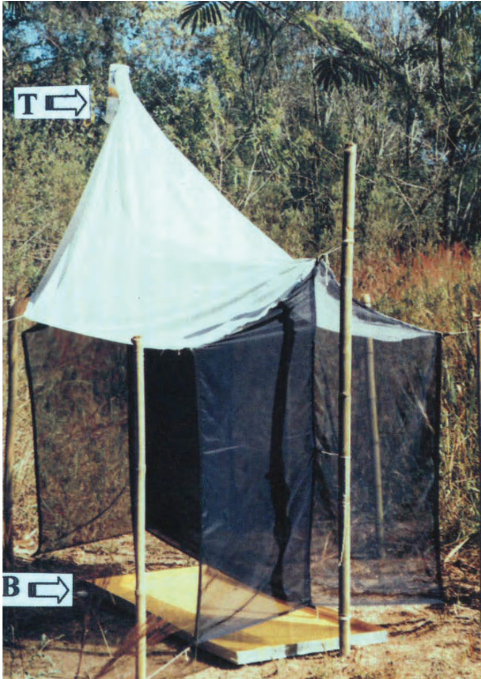
Fig. 34. Hybrid trap with the central diaphragm sprayed with insecticide and with a large yellow reservoir below it. T = top collector; B = bottom collector (From: Campos et al. , 2000)
