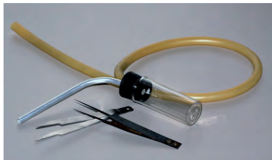
Fig. 1. Handling arthropods in the field. Delicate, soft bodied specimens can be handled with spring steel forceps. Minute, hard bodied specimens are best transferred by an aspirator which can be obtained from entomological suppliers. (Photo by authors).
