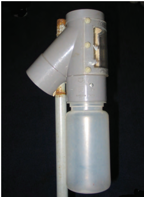
Fig. 6. Small grey PVC collector for Malaise trap (50 mm/45 degrees, 3.2 mm) with 0.2 l bottle. (Photo by C. van Achterberg).
