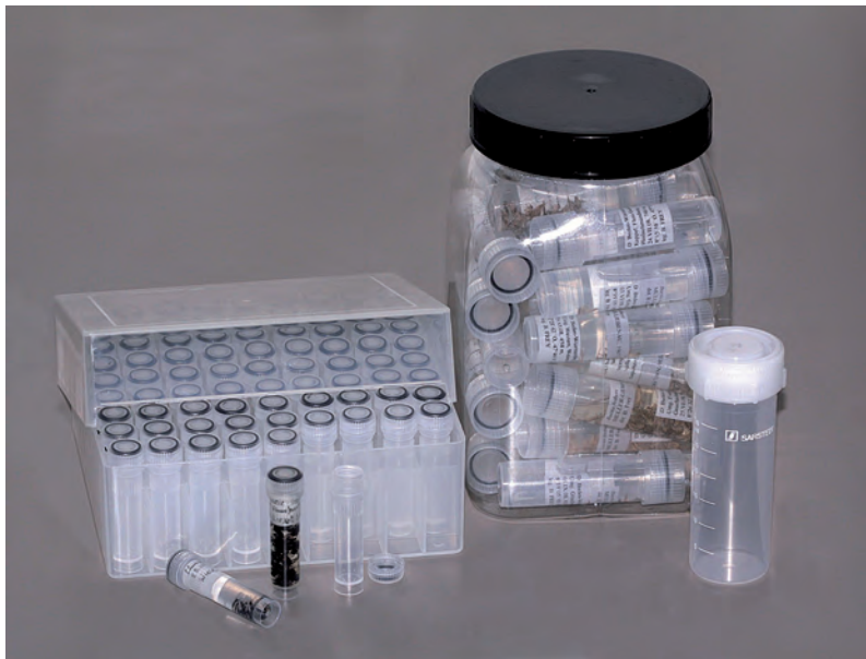
Fig. 3. Plastic vials are safer than glass vials during field work and also less heavy. A screw top with a ring gasket tightly closes the vials and prevents evaporation of the ethanol. The transparency of the vials allows the collector to check the content and labels without the need to re-open the vials. (Photo by authors).
