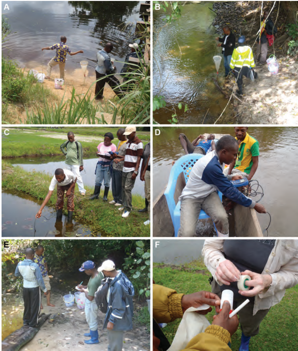
Fig. 13. Field collection methodology. A-B. Collecting samples with a phytoplankton net. C-D. Measuring of physical and chemical variables E-F. Taking notes in a field notebook and labeling of a sampling bottle.
